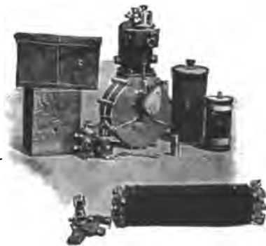
FIG. 306a.—A Typical Carriage Motor and its adjuncts: battery box and fuel tank; carburetor; cylinder on enclosed crank case; muffler; induction coil in gutta percha case; jacket water cooling radiator.
